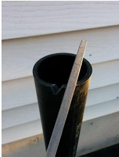
1. Cut your pipe to the required length (be sure the end is cut-off square and not at an angle). The length is up to you but should be long enough to do a full core of the normal maximum winter snow depth in your area. For most parts of Canada a length of 3 to 5 feet should be sufficient.
