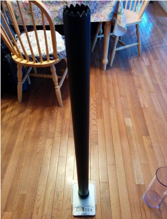
Bring your **2 inch** snow tube inside and place it on the scale. Be sure to first remove any snow or moisture on the outside of the tube:
