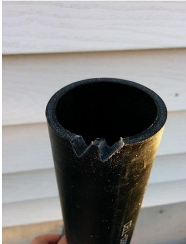
4. Begin the next cut for the 2<sup>nd</sup> tooth by using the full width of the file to measure the distance to the next cut in point.
