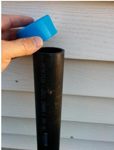
You will also need to purchase a blue plastic 2 inch Test Cap for the ABS pipe normally available in the same plumbing section of the store. A black ABS cap can also be used but is a bit more expensive and not required. The cap is required to keep your snow sample from falling out of the tube.
